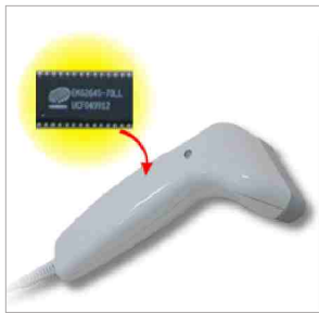
Embedded NeuroFuzzy decoding engine to read distorted barcode
